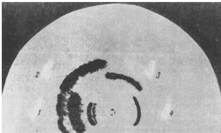
Fig. 2. Chromatogram of viridomycins A (2), B (3), and C (4) on paper in water-saturated ethyl acetate: 1) mixture of viridomycins A, B, and C.
